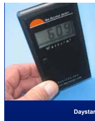
Figure 112. Handheld solar meters use a small PV cell to measure solar irradiance.
