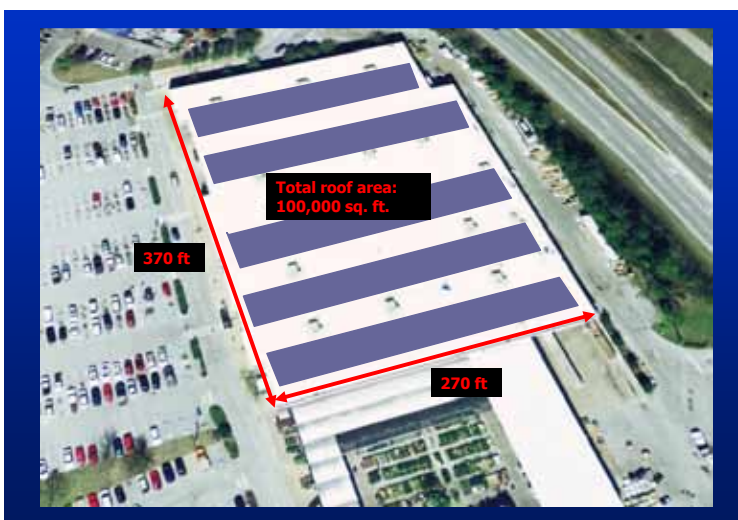
Figure 7. For a power density of 10 watts per square foot, a 500 kW PV array can be installed in a 50,000 square foot area.
