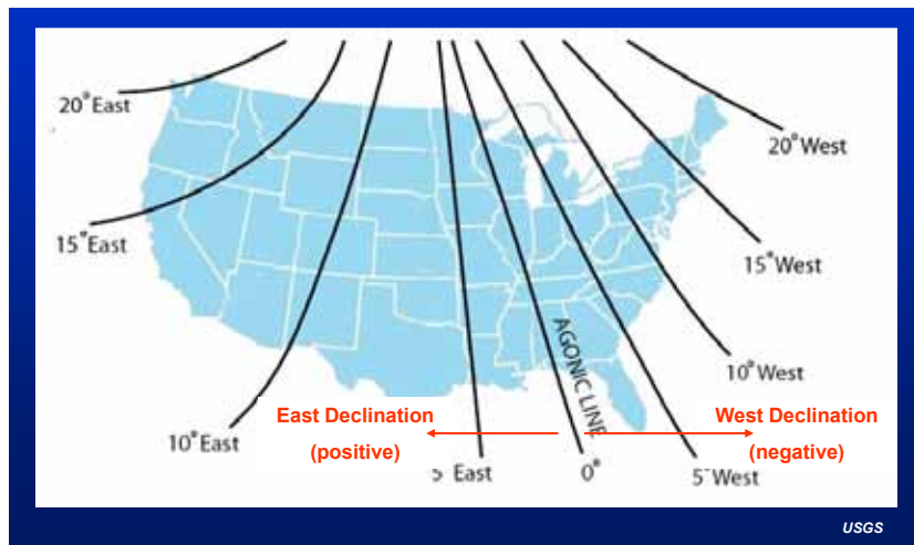
Figure 12. The western U.S. has positive (easterly) declination, and will cause a compass needle to point east of geographic north.
