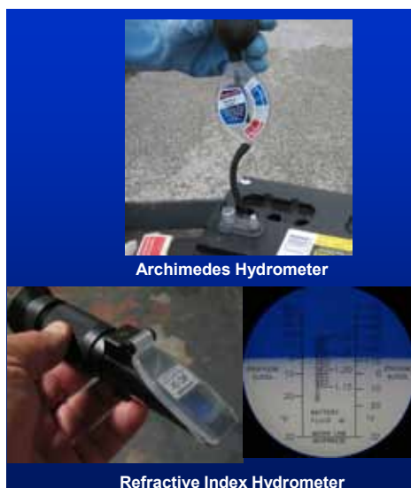
Figure 117. Hydrometers measure electrolyte specific gravity (SG).
