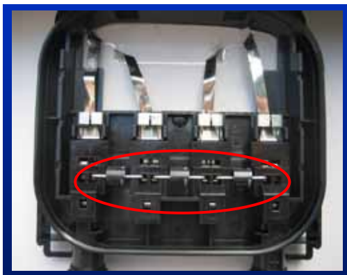
Figure 68. Bypass diodes are often located in module junction boxes.
