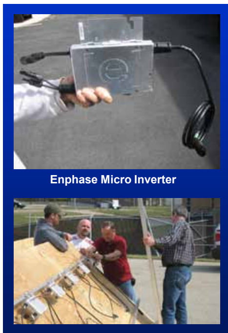
Figure 72. AC modules and micro inverters are small inverters installed integral to or adjacent to individual PV modules.
